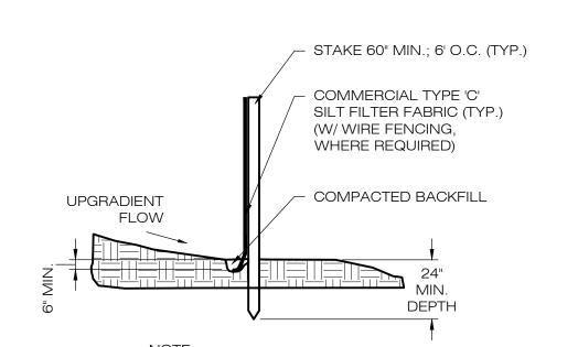
SILT FENCE SHALL BE LAPPED ONLY WHEN NECESSARY PER THE MANUFACTURER RECOMMENDATIONS.
