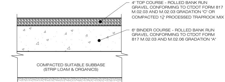
1. SUBBASE MAY CONSIST OF NATIVE MATERIALS IF FOUND ACCEPTABLE BY THE ENGINEER. SUBBASE TO BE COMPACTED TO 95% MAX DRY
