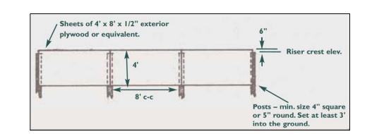
SEDIMENT TRAP BAFFLE SCALE: N.T.S.
