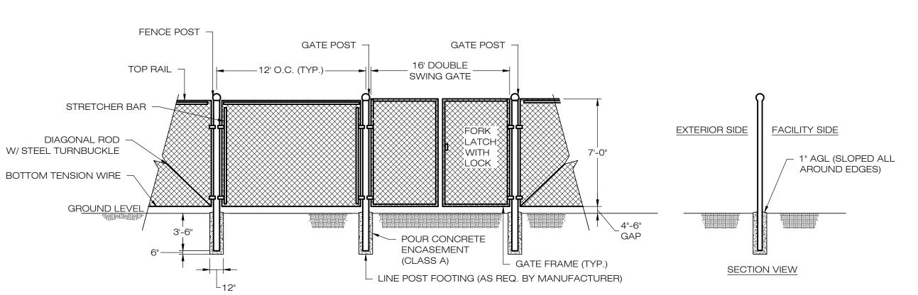
5 CHAIN-LINK FENCE & GATE DETAIL SCALE: N.T.S.
