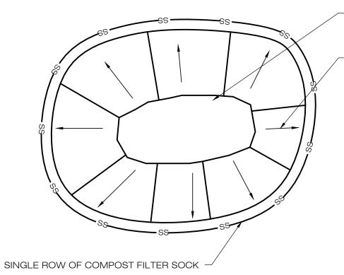
SOIL/AGGREGATE STOCKPILE OF EXISTING SITE MATERIAL TO BE REUSED AND/OR NEW MATERIAL TO BE INSTALLED IN THE WORK
