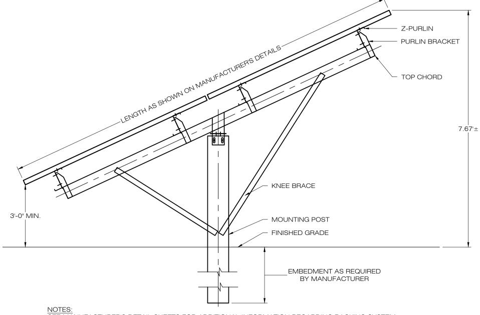
SEE MANUFACTURER'S DETAIL SHEETS FOR ADDITIONAL INFORMATION REGARDING RACKING SYSTEM REQUIREMENTS AND INSTALLATION PROCEDURES. RACKING SYSTEM TO BE INSTALLED IN ACCORDANCE WITH MANUFACTURER'S REQUIREMENTS.
