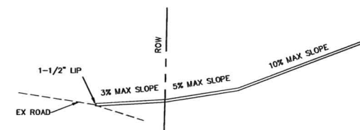
PROPOSED DRIVEWAY SECTION N.T.S.
