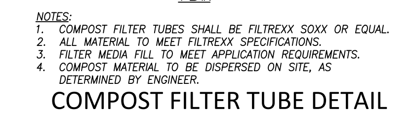
COMPOST FILTER TUBE DETAIL NOT TO SCALE
