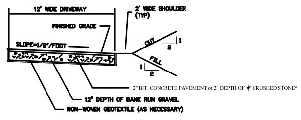
\* NOTE: 2" BIT. CONCRETE PAVEMENT REQUIRED WHERE SLOPE EXCEEDS 10%
