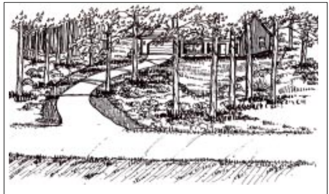
Figure 11. Site Fingerprinting Was Used on This Residential Lot to Reduce Clearing and Preserve Trees (PZC, 1992)
