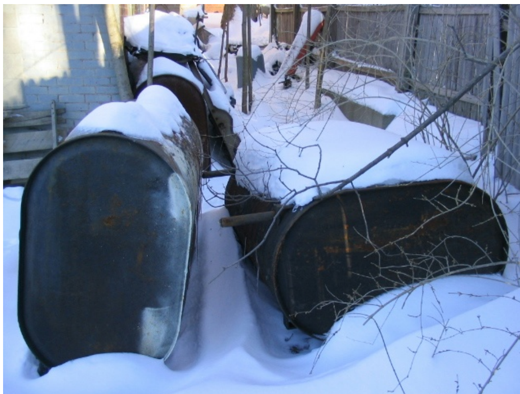
PHOTO: 06 LOCATION: Outside southern perimeter of property DESCRIPTION: Empty 300-gallon above ground storage tanks
